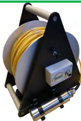
100m cable reel and camera head →
