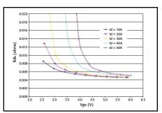
1µV measurement resolution and current sourcing up to 50A (100A with two units) enable low-level Rds measurements to support next-generation devices.
