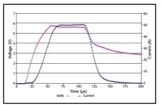
The dual digitizing A/D converters sample at up to 1µs/point, enabling full simultaneous characterization of both current and voltage waveforms.
