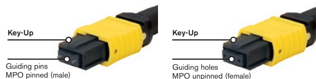
Figure 1: MPO and MTP male and female connectors
