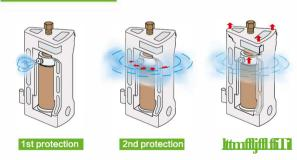
1si protection: pressure release via safety diaphragm 2nd protection: horizontal skirt-side pressure release 3rd protection: vertical pressure release
