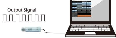
Note: When USG is connected to the PC, the signal is output at first. When software is activated, the output is set to OFF.
