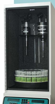
Cooling Carousel Racks protect and keep your samples cool during homogenization.
