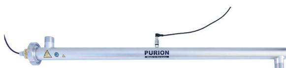
The UV-plant PURION 2500 36 W is made from electropolished stainless steel 1.4571. The PURION 2500 36 W is applied to disinfect drinking water up to a flow rate of 2.500 l/h and a transmission (or turbidity) of the water of at least 90% per cm.
