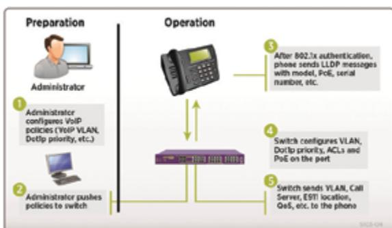
Figure 2: VoIP Auto Configuration with ExtremeXOS Universal Port
