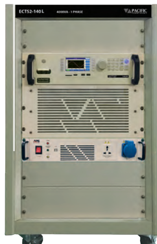
Single Phase 16A System for IEC 61000-3-2 and IEC 61000-3-3
