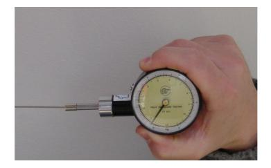
Our Fruit Firmness Tester (also known as a Fruit Pressure Tester) is a penetrometer that measures fruit firmness and provides a quick, easy and, according to university studies, accurate method to determine fruit maturity.
