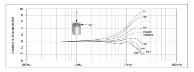
Free-field corrections for different angles of incidence
