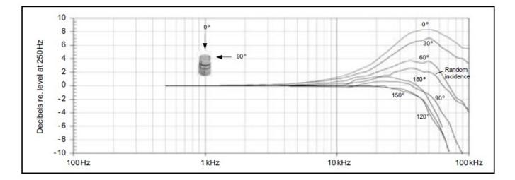
Free-field corrections for different angles of incidence
