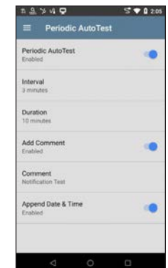
Periodic AutoTest enables monitoring infrastructure for intermittent issues
