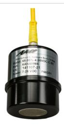
The AMI model 65 is the ideal solution for measuring oxygen in non-flammable gases in a general purpose environment. In a very small size, and at very low cost, it provides a basic electronic package with a single range voltage output (isolated current output optional) together with a zirconium oxide sensor that has an expected ten year life, with virtually no calibration required.
