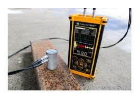
The electromagnetic-acoustic thickness gauge allows user to measure the thickness of metal products with one-side access without using couplant through a substantial gap (up to 6 mm). This significantly reduces the material- and laboriousness of the measurement process.
