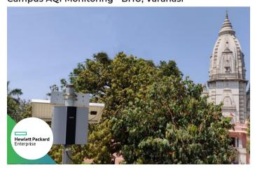
Oizom offered a comprehensive solution to help HPE monitor the environmental health of Banaras Hindu University and installed  $Polludrone^{^{TM}} \ in \ the \ campus. \ It \ monitored \ ambient \ air \ quality \ like$ particulate matter, gases and weather to aware the students. The solution showcased the data and also provided suggestive actions to help them take informed healthcare decisions based on AQI.
