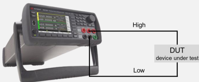
Same measurement using an SMU
