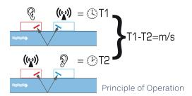
When ultrasound is transmitted between the transducers, its velocity is slightly increased when travelling in the direction of flow, and slightly reduced when travelling against the flow. The resulting transit time difference is directly proportional to the velocity of the flow in the pipe. Having measured the flow velocity and knowing the pipe cross-sectional area, the volumetric flow can be easily calculated.
