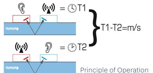
When ultrasound is transmitted between the transducers, its velocity is slightly increased when travelling in the direction of flow, and slightly reduced when travelling against the flow. The resulting transit time difference is directly proportional to the velocity of the flow in the pipe. Having measured the flow velocity and knowing the pipe cross-sectional area, the volumetric flow can be easily calculated.
