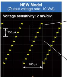
Oscilloscope settings: Band limit of 20 MHz, 16x averaging, auto-trigger
