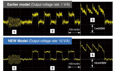
By improving voltage sensitivity of the oscilloscope by a factor of 10, the S/N ratio of the oscilloscope itself is enhanced to deliver a cleaner waveform.
