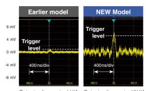
Output voltage rate: 1 V/A Output voltage rate: 10 V/A
