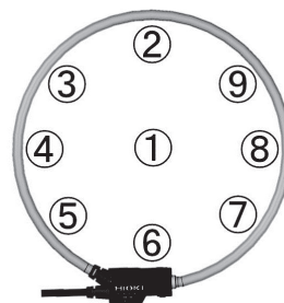
Fig. 14. Effects of conductor position: Measurement locations (ø30 mm conductor carrying 600 A at 60 Hz).
