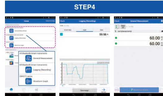
Return to the home screen and select a measurement function to display the corresponding measured values.
