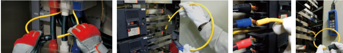
These sensors can be easily routed through confined locations and between cables. The tapered tip is designed so that it can be fed readily through tangled wires. In addition, a magnetic strap\* frees both hands for other tasks.
