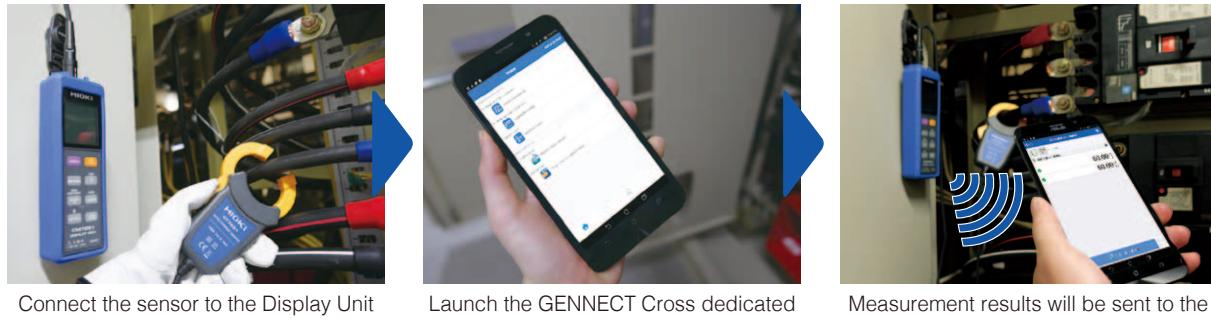
Connect the sensor to the Display Unit CM7291 and clamp in around the cable to be measured.
