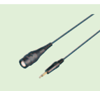
OUTPUT CORD L9095 Connect to BNC terminal, 1.5 m (4.92 ft) length, for the CM7290 or other
