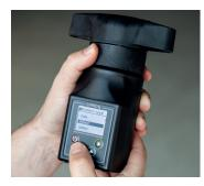
Turn on the device by pressing the power button and use the arrow keys to select crop type.
