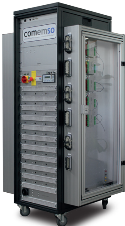
Full-Size BCS 3x 96 Cells for End-Of-Line Test
