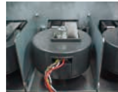
DCCT current sensor (in the PW3337)
