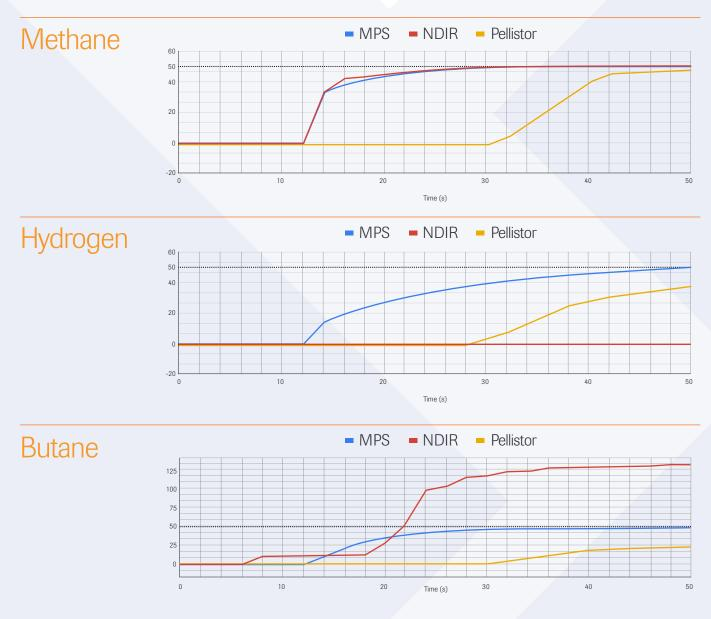
All 3 sensor types will react with the same output delivering an accurate reading for Methane (CH<sup>4</sup>).
