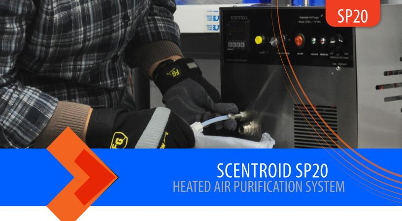
he Scentroid SP20 Heated Air Purification System is a revolutionary device designed to provide an effective and reliable cleaning solution for olfactometers, sample bags, PTFE lines, and other equipment which may be contaminated with odours.
