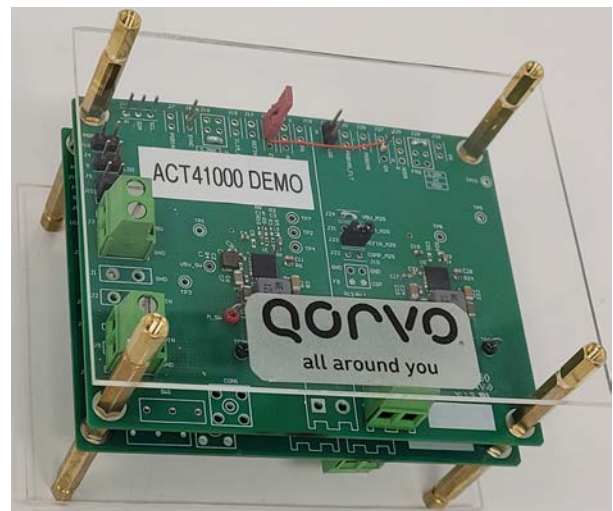
Figure 3. Four-Phase ACT41000 Reference Board
