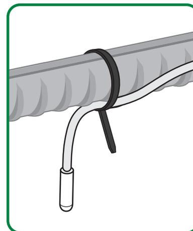
**6** Secure the cable and temperature probe below the rebar
