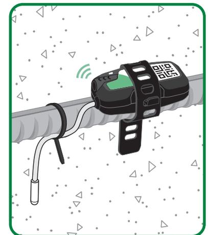
**7** Pour concrete and monitor results in the mobile app or remotely with SmartHub™
