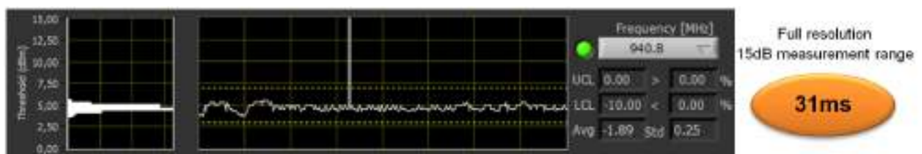
Real-time process monitoring by measuring the threshold power
