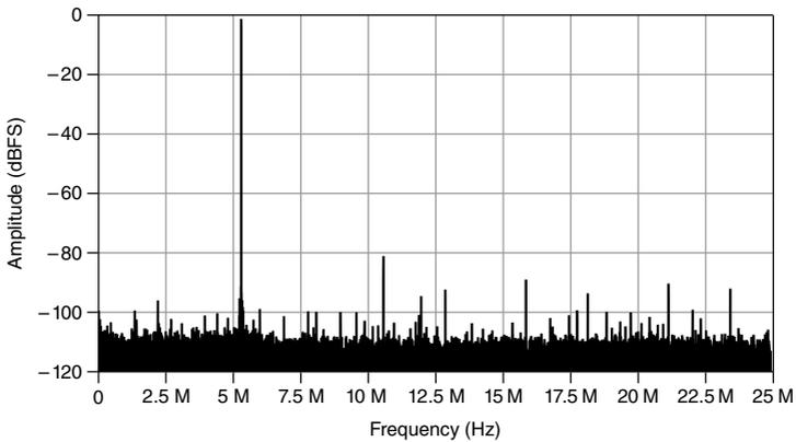
**Figure 4.** NI 5751 Characteristic Noise Density, Spectrum-64 k Samples
