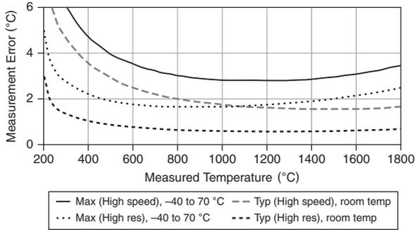
**Figure 6. Thermocouple Types R and S Errors**
