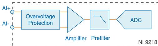
Input signals on each channel are buffered, conditioned, and then sampled by an ADC.
