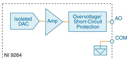
Each channel has a digital-to-analog converter (DAC) that produces a voltage signal. Each channel also has overvoltage and short-circuit protection.
