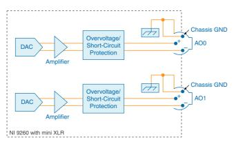
The output stage of the NI 9260 with mini XLR is balanced and fully differential. The AO- pin represents one output of the differential output driver and is capable of driving signals into the minimum load. Connecting this pin to GND will short circuit the output.
