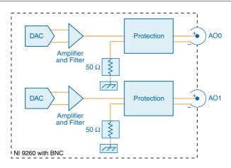
The Delta-Sigma DAC has a resolution of 24 bits and can update at a maximum rate of 51.2 kS/s. The output stage of the NI 9260 with BNC is pseudo-differential. AO- is terminated using a 50  $\Omega$  resistor to GND.
