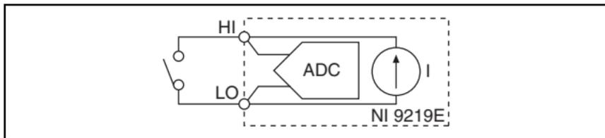
**Figure 13.** Connections in Open Contact Mode
