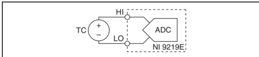
**Figure 12.** Connections in Thermocouple Mode
