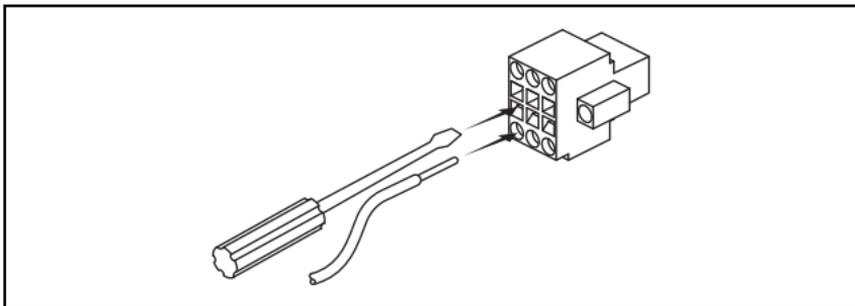
**Figure 3.** Connecting Wires to the NI 9219E Spring-Terminal Connectors
