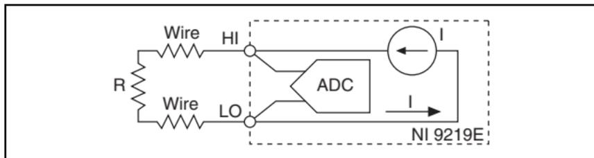
**Figure 10.** Connections in 2-Wire Resistance and Quarter-Bridge Modes
