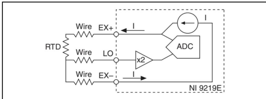
**Figure 9.** Connections in 3-Wire RTD Mode
