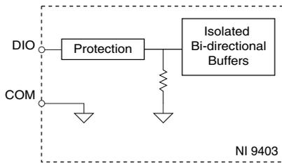
The DIO channels have Schmitt trigger inputs and are compatible with 5 V/TTL logic devices. Each input channel has hysteresis for improved performance with noisy and non-monotonic input signals. Each channel also has a pull-down resistor.
