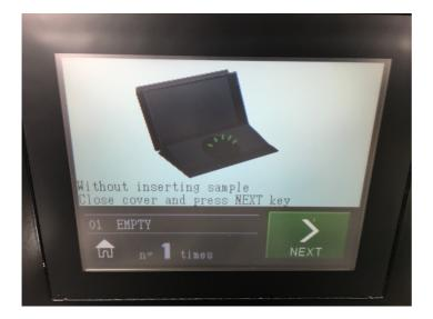
Take a reference measurement without a sample.  $\downarrow$ Insert a sample, and press [NEXT].  $\downarrow$ Rotate the sample front to back (180°), then press [NEXT].  $\downarrow$ Sampling complete. <6> Sampling of No. 1 data is complete.
