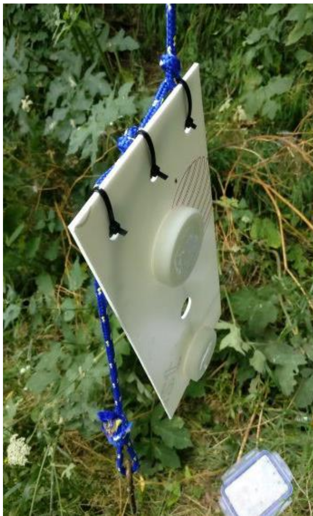
Figure 7: Chemcatcher® plastic plate with 2 Chemcatchers in place
