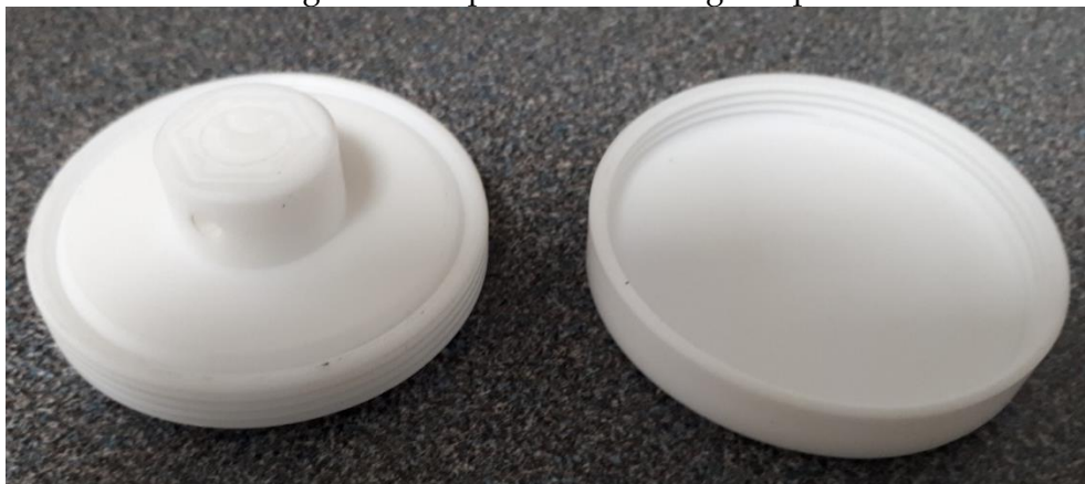
Figure 2 Supporting Disk (screwed into retaining ring) and transport lid
