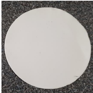
Figure 5 Membrane 47mm (type depends on target compound to be monitored)
