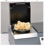
It is used for measuring the samples that will not fit into the Petri dish supplied as an accessory. The light shielding cover can be used as well. Therefore, it is applicable for the samples whose light transmittancy is high.
