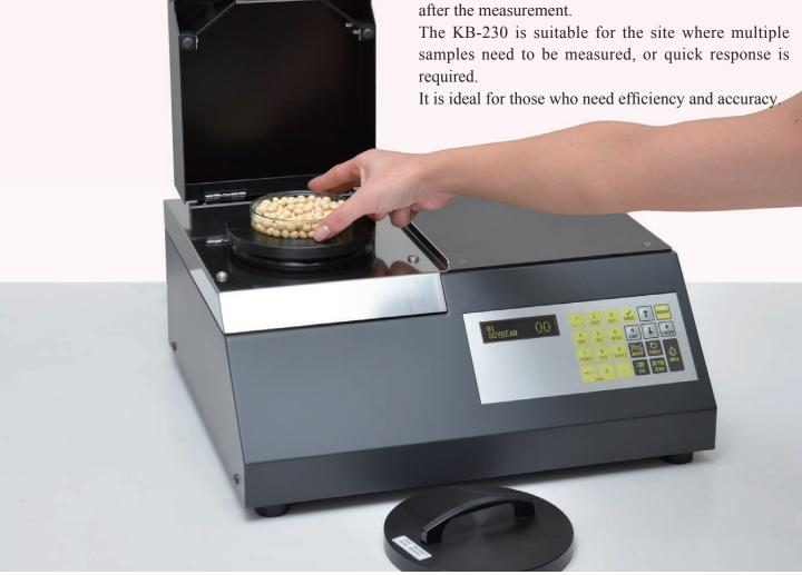
Conventionally, the near-infrared is emitted at the top surface of the sample. In this method, how you can make the surface of the sample flat affected the measurement.
