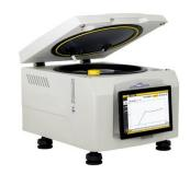
professional software which supports automatic controlling of temperature, humidity and flow rate precisely and guarantees the testing sensitivity and repeatability of the test results. C360M is applicable to determination of water vapor permeability of plastic films, sheeting, paper, packages and other packaging materials in food, pharmaceutical, medical apparatus, building materials and consumer goods, etc.
