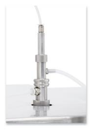
The spray assembly incorporates an automatic de-blocking device that prevents the jet nozzle from becoming blocked, the de-blocking needle is activated by an integral compressor. De-blocker is sometimes necessary with materials which may solidify or when large particles in suspension cause blockages in the jet.
