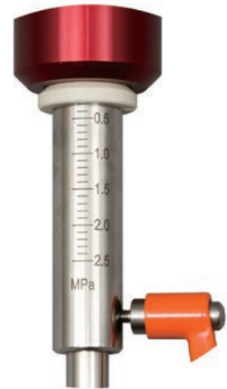
Scale part (Measurement range 0 - 2.5MPa) / Enlarged view
