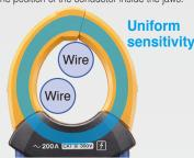
Zero-phase current can be accurately measured since the meter is resistant to the effects of conductor position.
