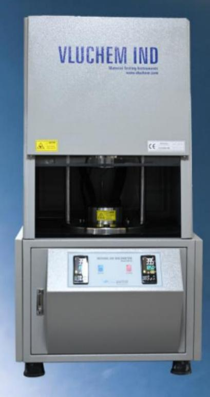
The Vluchem's moving die rheometer (MR-10) for determining selected vulcanization characteristics of vulcanizable rubber compounds using rotorless sealed torsion meter and measured according to ASTM D 5289, ISO 6502-3 and KS M ISO6502.
