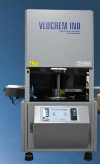
The Vluchem's automatic moving die rheometer (AMR-10) for determining selected vulcanization characteristics of vulcanizable rubber compounds using rotorless sealed torsion meter and measured according to ASTM D 5289, ISO 6502-3 and KS M ISO6502.
