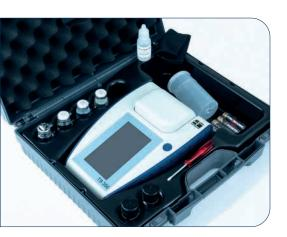
Take it or leave it: The TB350 turbidity meter is ideal for portable use in field applications such water distribution systems monitoring and laboratories that test a wide range of samples.
