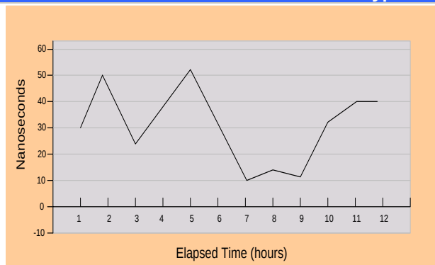
Typical time error fluctuations when disciplined to GPS
