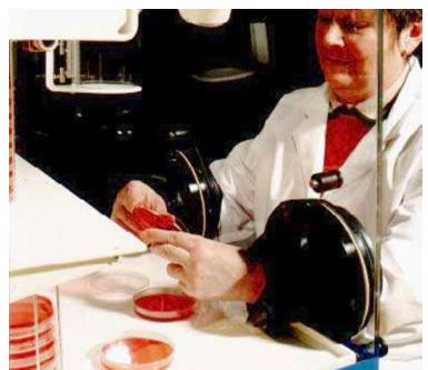
**Glove Free Operation:** This unique bare hand method is very simple to operate. Air-tight seals fit around the user's wrists as shown and the anaerobic atmosphere is maintained. The design eliminates the use of footswitches and gets rid of large internal arm port bungs, giving more working room inside the incubator. The system is very economic on gas usage and the hands can be inserted in seconds.
